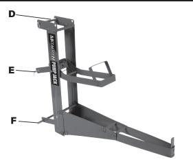
Attach the pump jack to the pole with the bed facing the work wall, by removing pin and roller (**D**) crank (**E**) square rod (**F**). Place the pump jack over the pole and reconnect parts.
