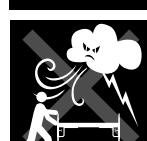
NE PAS UTILISER L'ÉCHAFAUDAGE PAR MAUVAIS TEMPS OU PAR GRAND VENT
