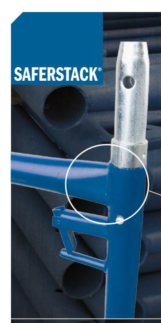
At Metaltech<sup>®</sup>, we innovate to make your life easier and safer. We have redesigned the standard frame to maximize the stacking height of a pile by flattening the horizontal tubes diameter from 1.69" to only 1".
